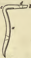
Fig. 42. Butt-plate and screws, quarter size, three views. a , body; b , toe; c , heel; d , d , screw-holes; e , e , screws.
